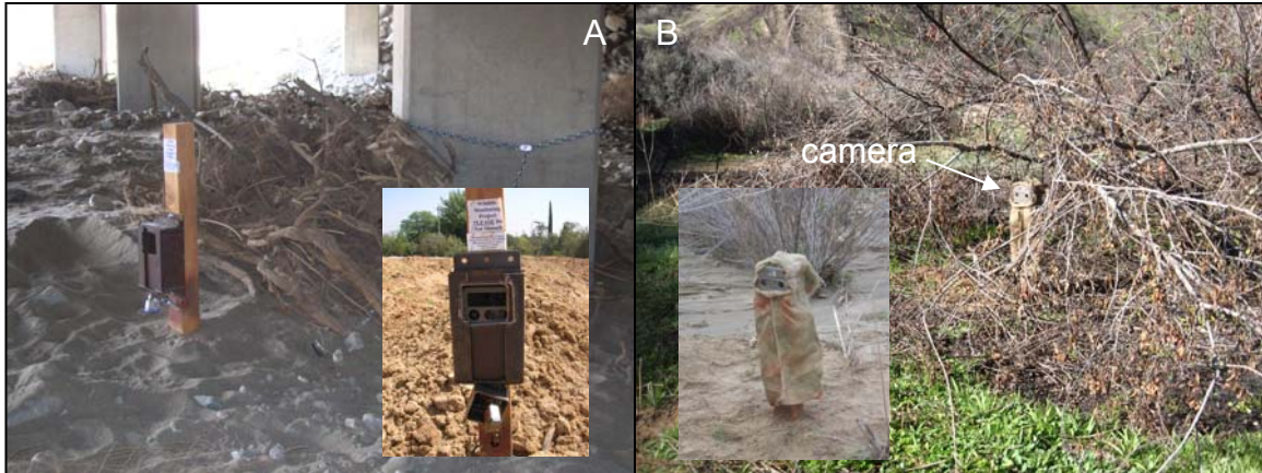
Figure 4. Camera station designs for units placed under bridges with steel box and chain(A), and cameras deployed without steel box and concealed with burlap (B).
